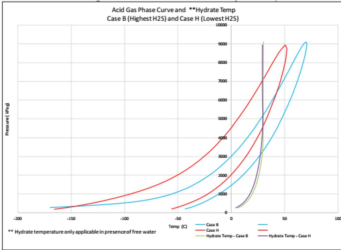
Hydrate curve includes the points where hydrates might form but is based on the presence of free water. The disposal stream typically do not contain free water, but if the well was flowed back, it may contain free water from the formation – depending on the dessicant significance of the disposal operations. Longer term disposal with higher volumes would likely result in a water-free area around the wellbore due the dessicant properties of the disposal stream.
