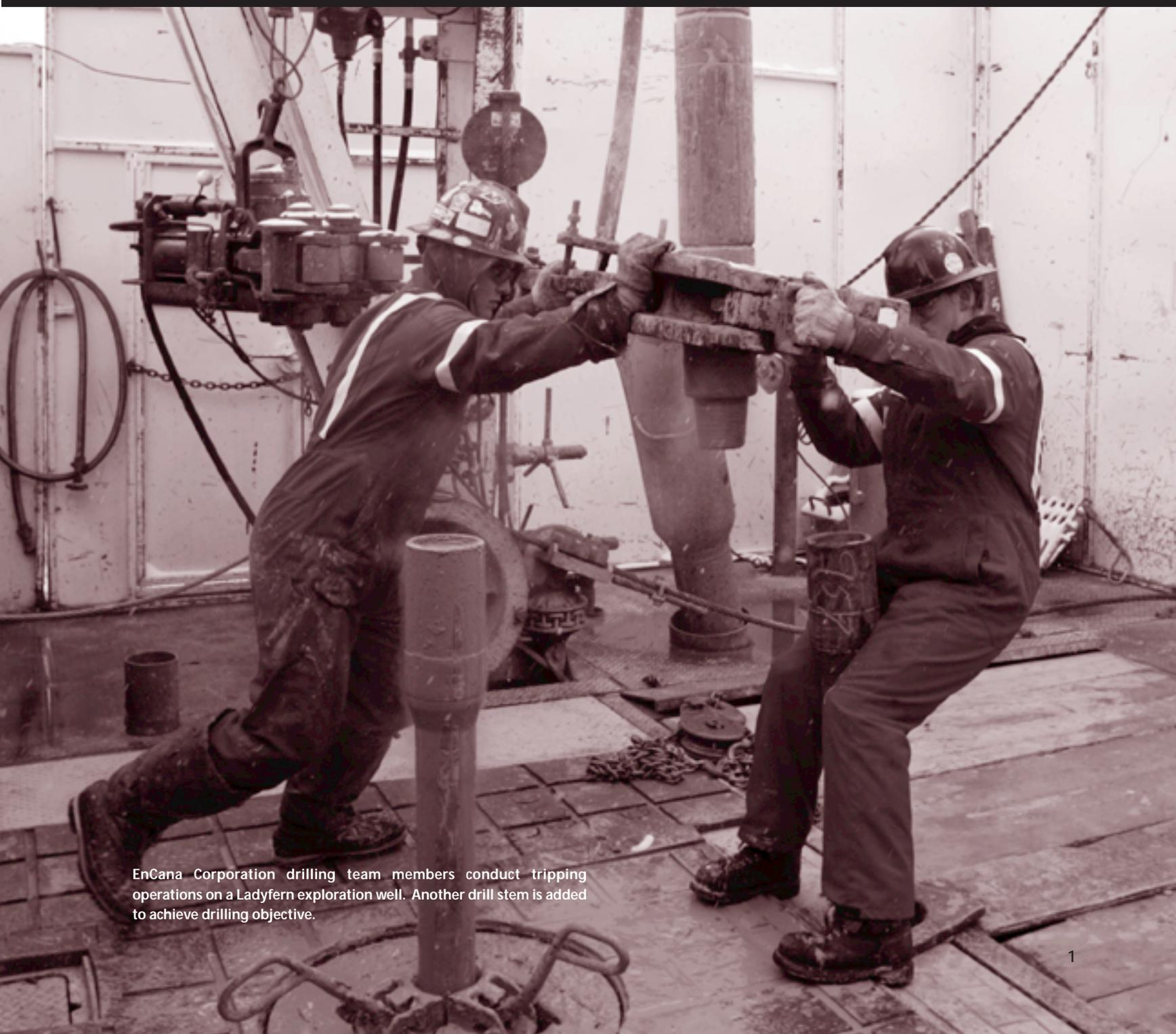
EnCana Corporation drilling team members conduct tripping operations on a Ladyfern exploration well. Another drill stem is added to achieve drilling objective.
